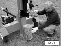
e. Only using your hand, push the control lever down (towards the log). If the log moves before it is contacted by the splitting wedge, release the control lever and then reposition the log. Operate the log splitter only when standing in the safe operating area, as shown in the picture.
