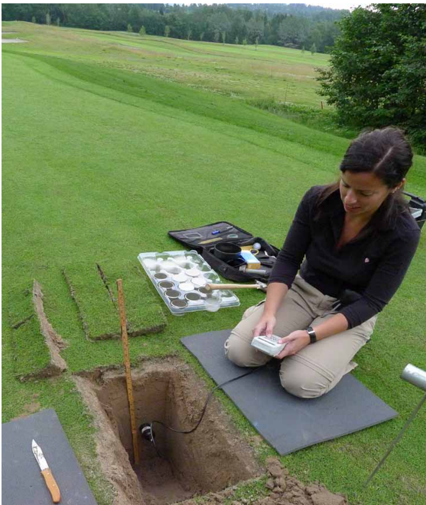
Photo 3. The soil water content increases towards the gravel layer on USGA greens. Photo: Agnar Kvalbein.
