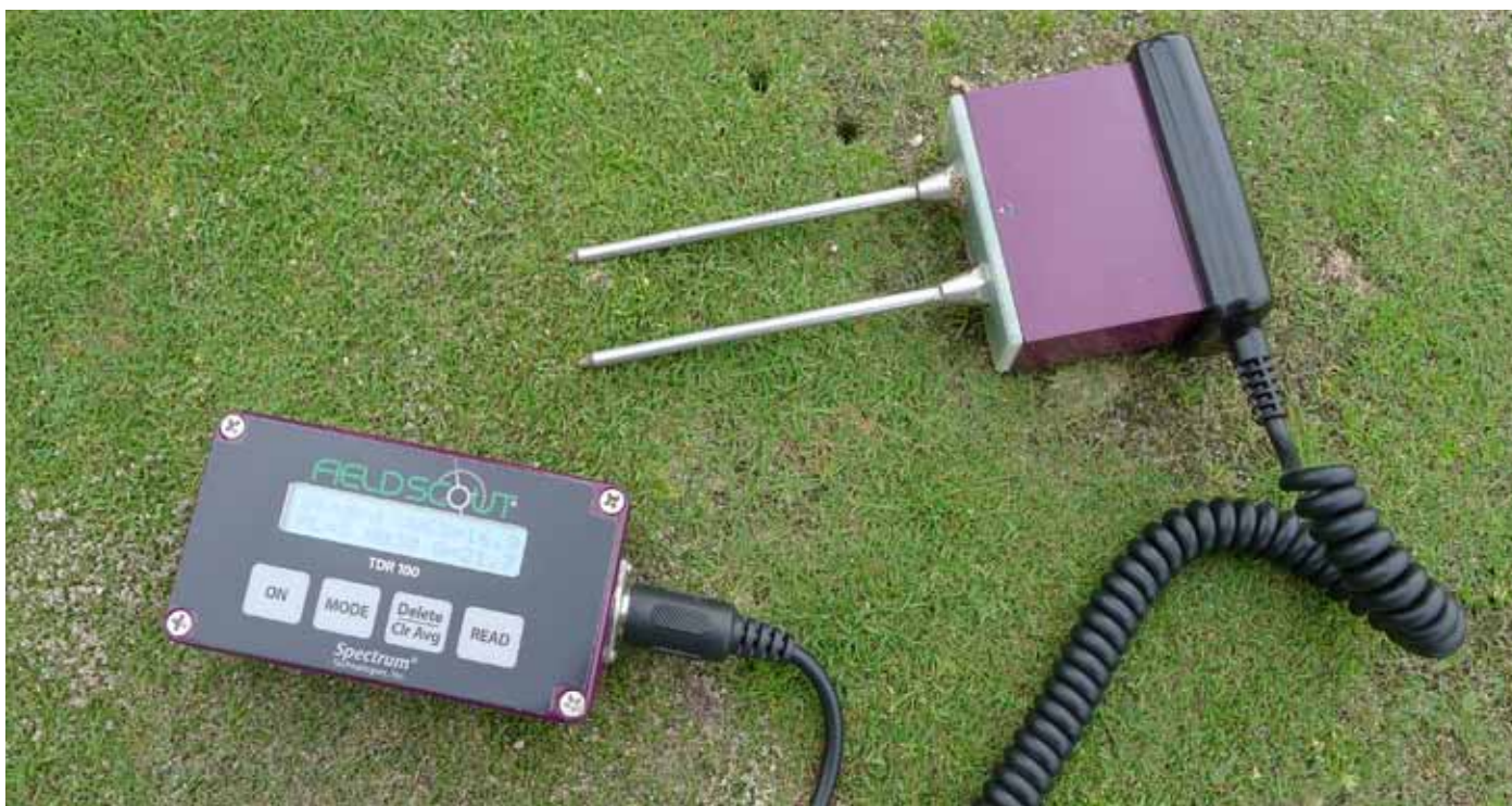
Photo 10. Time Domain Reflectometry (TDR) instrument used to measure volumetric soil water content. Photo: Agnar Kvalbein.
