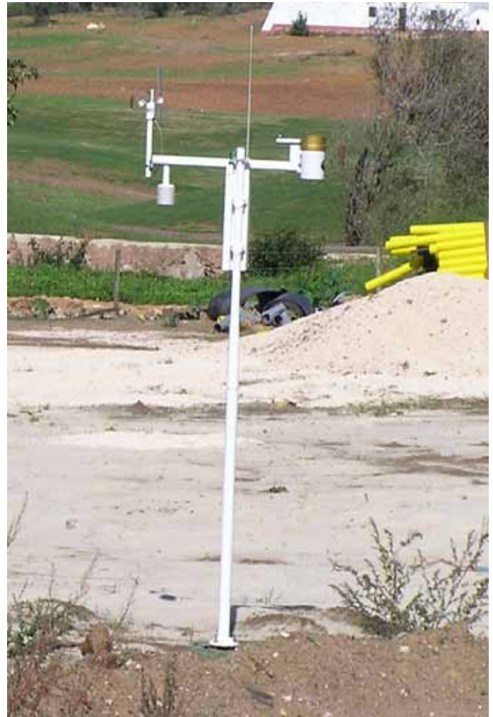
Photo 5. A weather station that calculates ET_0 from temperature, solar radiation, wind speed and relative humidity can be connected to the irrigation system (Photo: Agnar Kvalbein).
