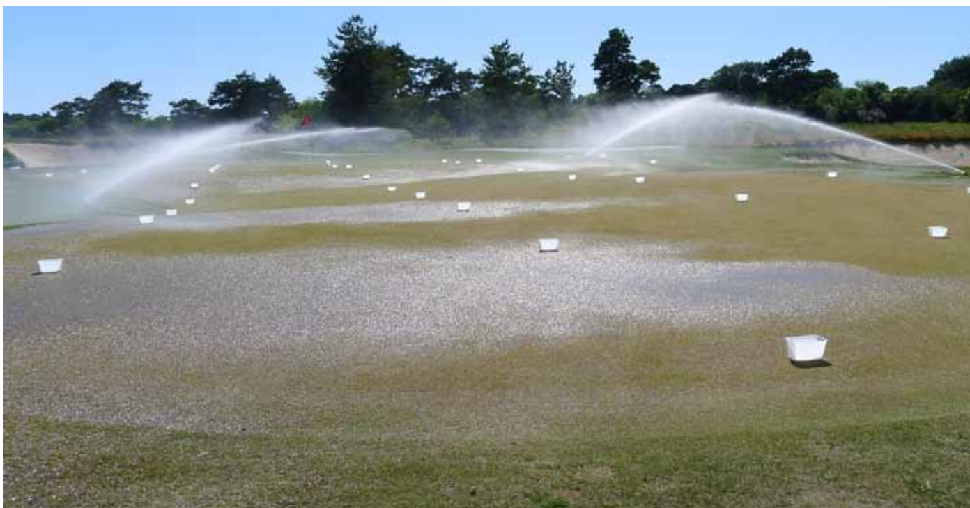
Photo 11. The intensity of a modern irrigation system is often higher than the infiltration capacity. On undulated greens this will result in uneven distribution of water even if the sprinklers are correctly placed and well maintained. This photo from Visby GC, Sweden, shows water ponding in lower areas during a distribution uniformity test. Photo: Agnar Kvalbein.
