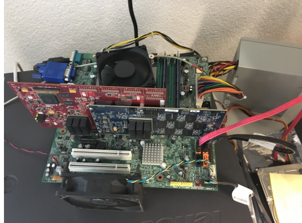
Figure 2: Evaluation testbed: green, red, and blue PCBs are the server motherboard, Gateway and CPU board, and FPGA and NAND Flash board, respectively.
