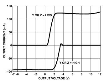
FIGURE 10. DRIVER OUTPUT CURRENT VS SHORT CIRCUIT VOLTAGE
