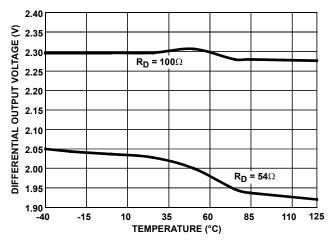
FIGURE 9. DRIVER DIFFERENTIAL OUTPUT VOLTAGE vs TEMPERATURE
