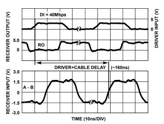
FIGURE 16. DRIVER AND RECEIVER WAVEFORMS DRIVING 100  $^{\circ}$  (31m) OF CAT5 CABLE (DOUBLE TERMINATED WITH 120 $\Omega$ )
