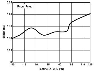
FIGURE 13. DRIVER DIFFERENTIAL SKEW vs TEMPERATURE
