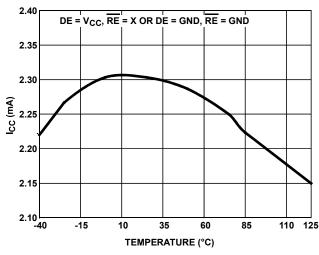
FIGURE 11. SUPPLY CURRENT vs TEMPERATURE
