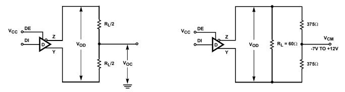
FIGURE 1A.  $V_{OD}$  AND  $V_{OC}$
