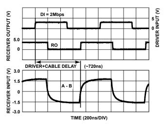
FIGURE 17. DRIVER AND RECEIVER WAVEFORMS DRIVING 500' (152m) OF CAT5 CABLE (DOUBLE TERMINATED WITH 120 $\Omega$ )
