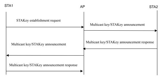
Figure 43ag—The flow chart of the STAKey establishment
