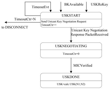
Figure 43at—Authenticator state machine, Part 2
