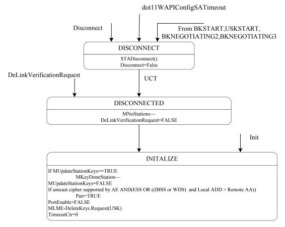
Figure 43au—Authenticator state machine, Part 3
