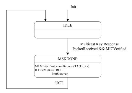
Figure 43ar—Supplicant state machine, Part 2
