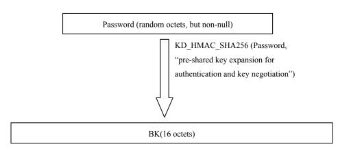
Figure 43am—Preshared key derivation architecture
