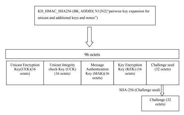
Figure 43ak—Unicast key derivation architecture
