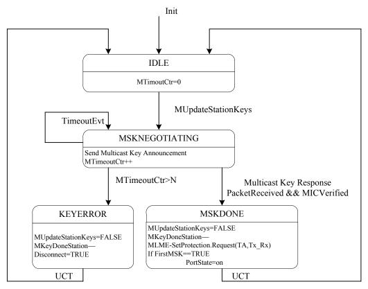
Figure 43av—Authenticator state machine, Part 4
