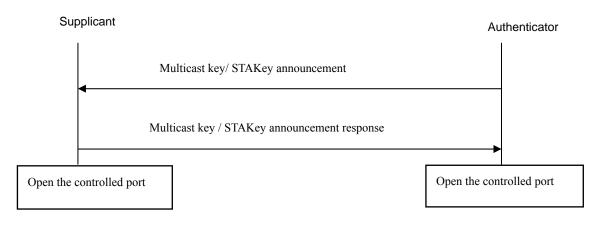
Figure 43ad—Multicast key / STAKey announcement procedure
