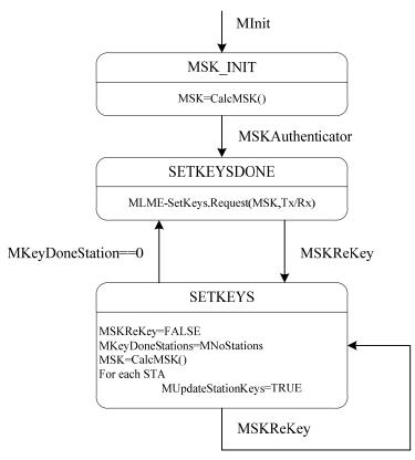
Figure43aw—Authenticator state machine, Part 5
