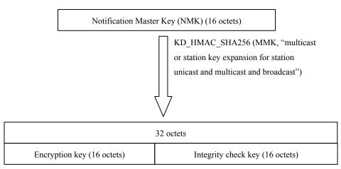
Figure 43al—Multicast / STAKey derivation architecture
