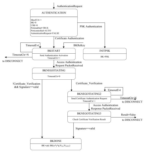
Figure 43as—Authenticator state machine, Part 1
