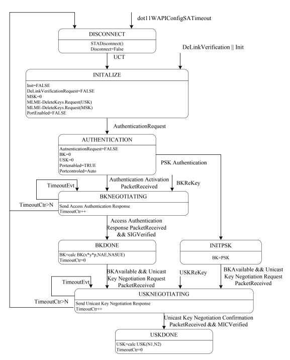
Figure 43aq—Supplicant state machine, Part 1
