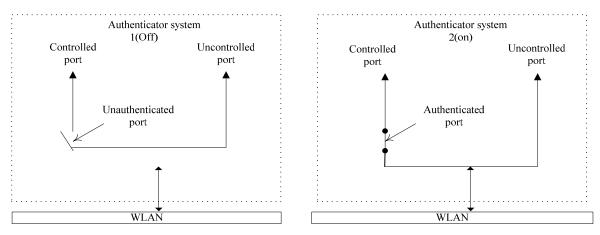
Figure 43b—Authentication state on controlled port
