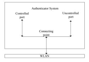
Figure 43a—Uncontrolled and controlled ports
