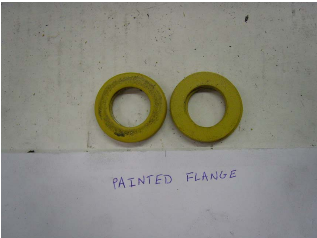
Figure 8 – Test Series 1 Post 3 rd Bolt-up Washer-Flange Faces
