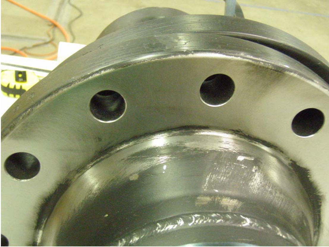
Figure 9 – Test Series 2 Paint removed from flange
