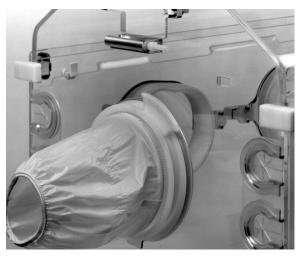
b. Fold back, and slip the larger elastic band over the outer ring of the port housing.
