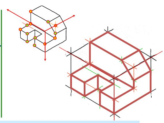
**Note** In isometric sketch/drawing), hidden lines are *omitted* unless they are absolutely necessary to completely describe the object.
