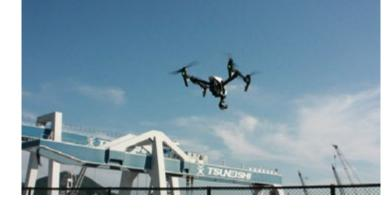
At the International Association of Classification Societies (IACS), discussions on the use of Remote Inspection Techniques (RIT) including drones in class surveys are already underway, and IACS Rec. 42 (Guidelines for Use of Remote Inspection Technics for Surveys) was revised in June of 2016. A revision of the related IACS Unified Requirements has also been completed and will take effect in January 2019.
