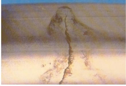
Figure 6 - Stress corrosion cracking of 316 stainless steel
