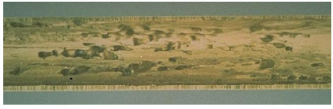
Figure 3 - Erosion corrosion of 90-10 copper-nickel when exposed to excessive flow rates
