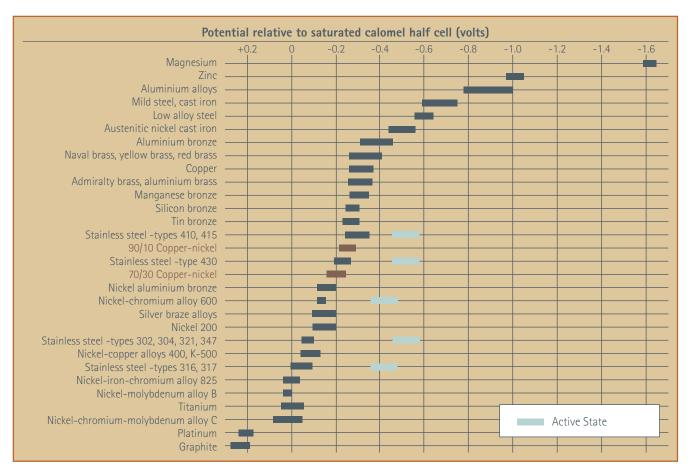
Figure 7 - A galvanic series in seawater(2)
