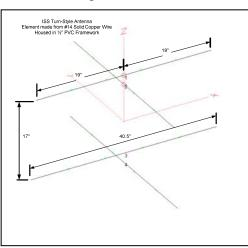
The actual antenna elements are made from common #14 electrical wire available at home improvement stores (insulated or non-insulated). The simple wires are not rigid enough to maintain their shape as an antenna; therefore, the antenna elements are inserted into an exoskeleton made of common ½ inch PVC pipe. The PVC exoskeleton is connected together with simple PVC fittings.
