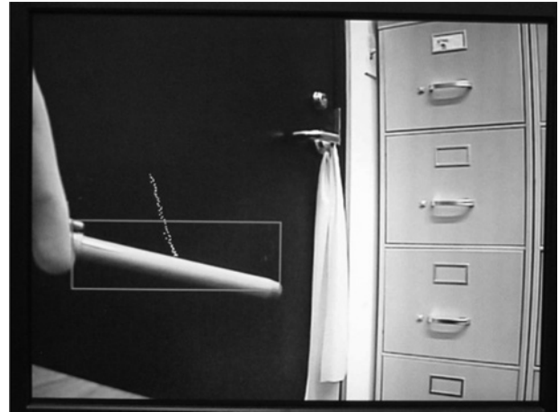
Fig. 18 Real-time video output shows a green pen framed by a rectangular box
