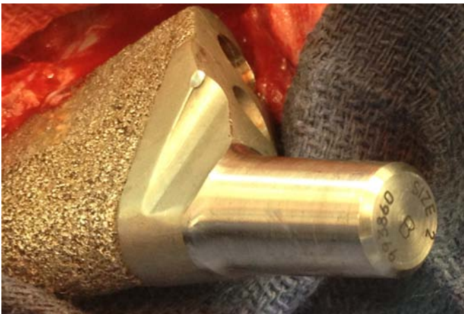
Figure 8. Intra-operative photograph of modular taper junction of the femoral stem. The ceramic head did not have an internal metal jacket. The taper junction shows no abnormal abrasion and is free of corrosion.
