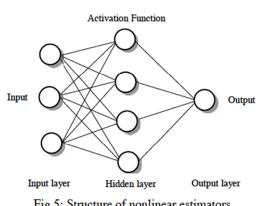
Fig.5: Structure of nonlinear estimators
