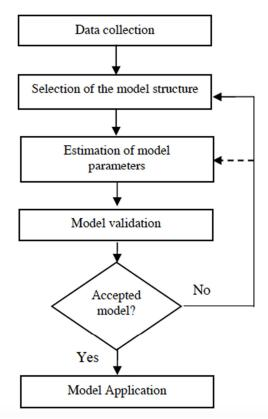
Fig 1 . Process Of System Identification
