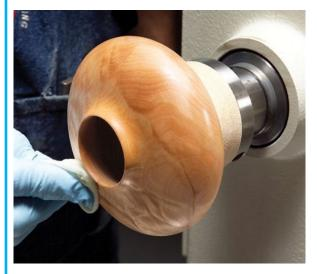
French polish adds extraordinary depth to gorgeous wood. This finish is perfect for bowls, vessels, lamps and other turnings that aren't handled often or are exposed to moisture, alcohol or heat. It's easy to apply: Just hold a cloth moistened with the finish directly to your project as it spins on the lathe.
