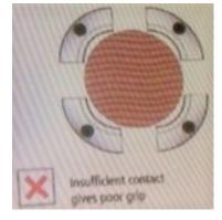
Insufficient contact gives poor grip
