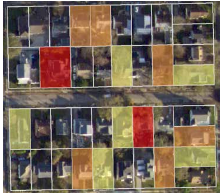
Figure 4: Tax parcels with highest volume of change shown in red, moderate changes - orange, slight change - yellow. Parcels with NULL color indicate that the changes detected fell below the user defined threshold.
