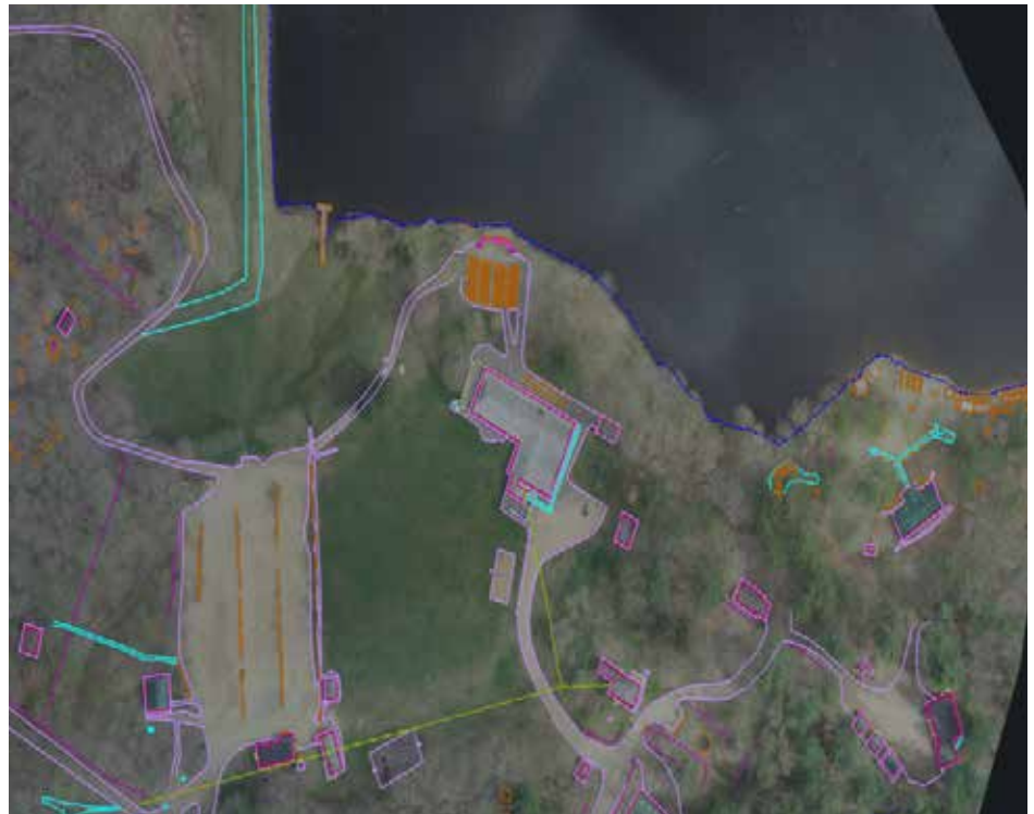
Figure 6: Digitized Data from Orthoimagery (Portion)
