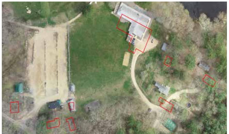
Figure 3: The shift of LiDAR data with Initial Orthoimage
