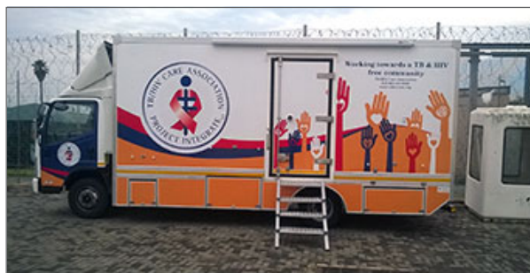
The mobile X-ray clinic built on an FAW 8.140 FL chassis cab.
