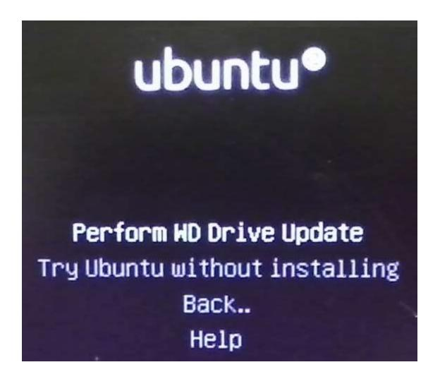
At this screen, make sure **Perform WD Drive Update** is highlighted, then press **Enter** to continue loading Linux. If **Perform WD Drive Update** is not highlighted, press the up or down arrow until it is highlighted, then press **Enter**.
