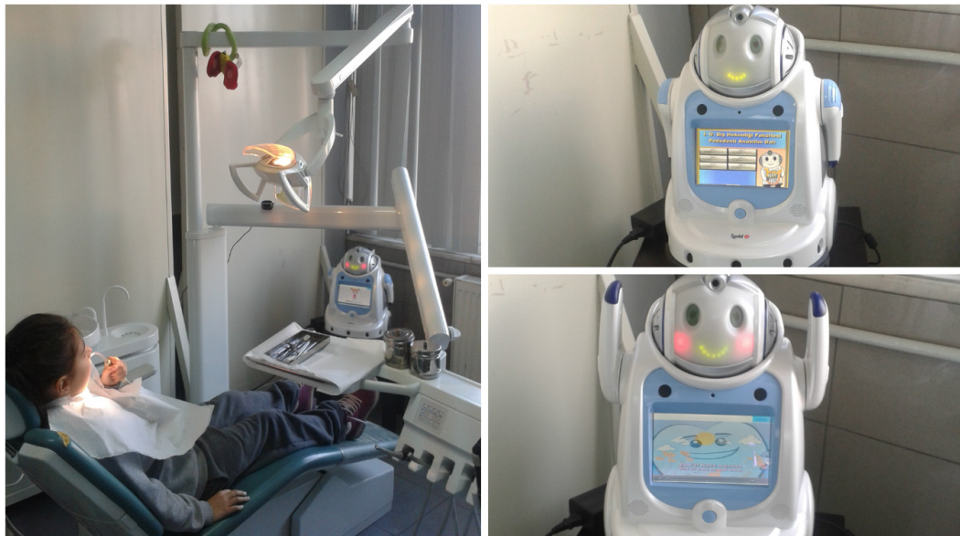
Figure 4.4 : IRobiQ performs some body movements with face expressions during a child's dental treatment.
