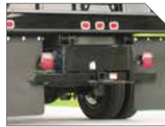
COMBINATION CLASS V HITCH AND ICC BUMPER*
