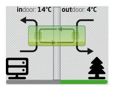
Indirect means that a heat transfer media is used between ambient air and the Data Center
