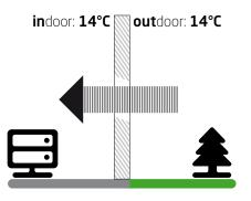
Direct means that ambient air is used directly to remove heat load gnerated by IT equipment **Pros**: More efficient **Cons**: air quality issues, humidity control.
