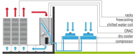
Direct expansion systems equipped with free cooling coils, to be connect with external dry coolers, are an effective and efficient solution for small to medium data rooms, where the installation of large external chiller is problematic and when it is anyway take advantage of favorable climate conditions.
