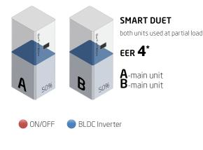
\*thermal load 23 kW at 24°C/50% rh internal conditions and 35° outdoor conditions
