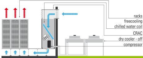
A direct expansion system with direct air free cooling is definitely the most efficient solution as it profits from the most favorable conditions of outside air that may occur during the year. Ideal for rooms with high turnover equipment, where outside air immission is not considered problematic and humidity control inside is not too stringent.
