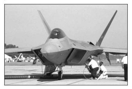
The F-22 is powered by twin Pratt and Whitney F119 turbofan engines rated at 35,000 pounds of thrust apiece. These engines allow the Raptor to reach a supersonic cruising speed of Mach 1.58 without the use of afterburner.
