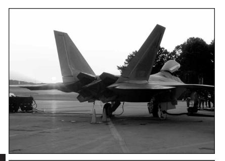
The F-119 engines feature a two-dimensional thrust vectoring system. Horizontal fins at the exhaust deflect thrust plus or minus 20 degrees. This gives the Raptor is superior agility in combat.
