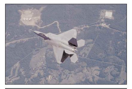
The F-22 has been designed with stealth as a primary goal. Composed primarily of titanium, thermoplastic composites, and radar absorbent materials, the F-22 is both lightweight and strong.
