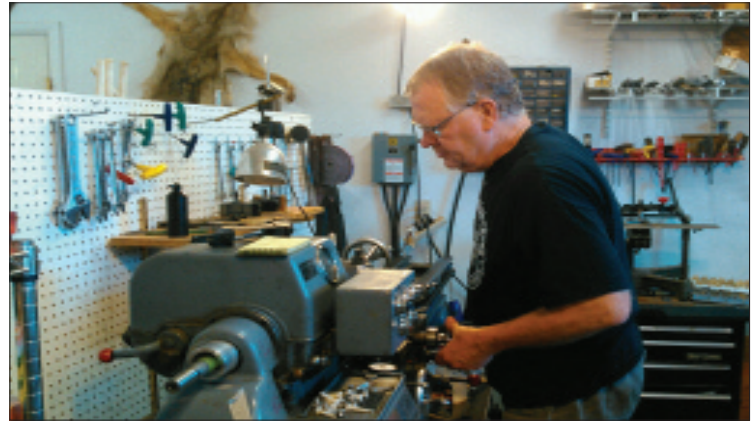
Pat Knight Threading Barrel At The Lathe
