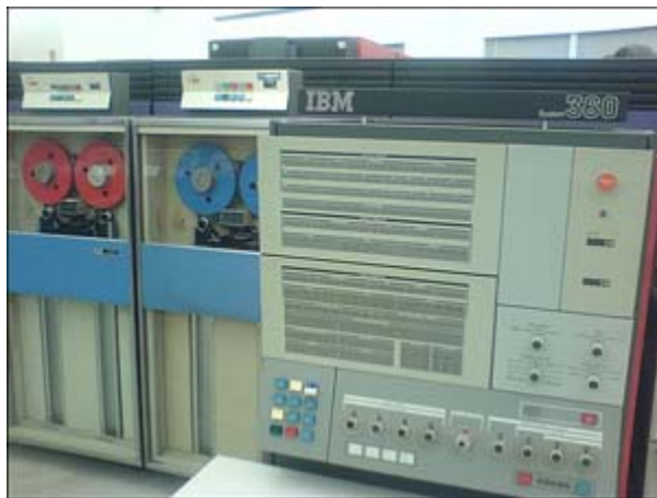
Figure E-2. Operator Console of IBM System/360 (Reprint Courtesy of International Business Machines Corporation, copyright International Business Machines Corporation)
