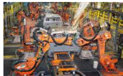
Chrysler Warren Truck Assembly Plant, Dodge Ram Box line, Body in White
