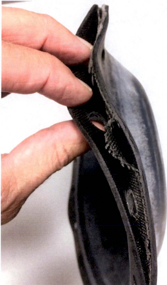
Figure 2: Delamination of fabric from elastomer
