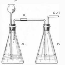
Fig. 7. The simplest gas-generating apparatus is made from two flasks (A) and (B) carrying two-holed stoppers through which passes the thistle tube and glass tubes as shown.
