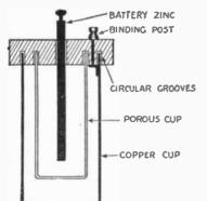
A slight departure from the conventional type makes an efficient portable Daniel cell for experiental uses
