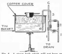
Fig. 6. A steam bath which will not burn out. A strip of paper placed in the bottom of the con-tainer will char and attract the experimenter's attention, however, if the water does evaporate completely.
