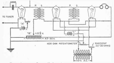
The experimenter may dispense with the cumbersome storage battery by employing a toy transformer shunted by a potentiometer for lighting the amplifier tubes. Note that a  $1\frac{1}{2}$ -volt dry cell tube is used for the detector with separate "A" battery in order to eliminate the A. C. hum.
