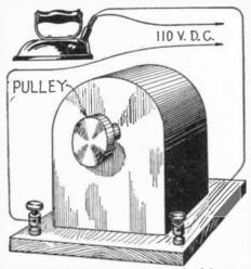
A handy high-speed motor for the laboratory constructed from a discarded automobile generator. A flat-iron acts as a resistance.
