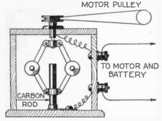
A centrifugal governor, varying the length of a carbon resistance connected in series with the electric motor. The motor turns the governor; practically constant speed is attained.
