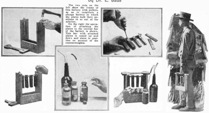
The mixing of the solution using a medicine measure or graduate and an extemporized wash bottle, are shown directly above and the portability of the battery and its great convenience are shown by the figure carrying it like an ordinary bundle.
