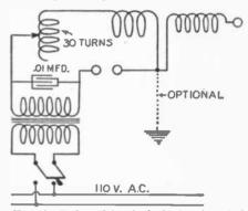
How the Tesla coil is wired, the location of the spark-gap and condenser and the optional grounding.
