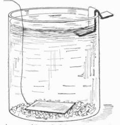
A copper sulphate cell of the gravity type; constant, but if left on open clrcuit the zinc becomes coated with copper.
