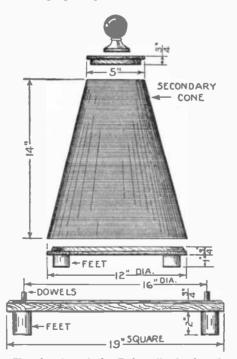
The elevation of the Tesla coil, showing the cone wound with wire and the circular base with its supporting feet and dowels.
