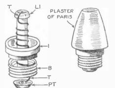
A resistance made from a burnt-out fuse, lead-in or tubular insulator. A nichrome wire is wound around this and the whole is then set in plaster of Paris. The brass thread of the original plug is utilized.
