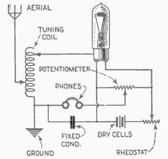
The connections of the two-element tube are clearly shown. By careful adjustments of the potentiometer and rheostat exceptional sensitivity is obtained. Note how simply this tube may be adapted to the standard crystal circuit. ments of the old crystal set with the exception of the crystal. The rheostat is
