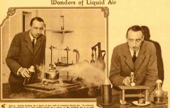
Above. Kettle boiling on a lump of ice, only it contains liquid air. It presents the appearance of a very active kettle on a stove, as the gasified air is so cold that it produces a cloud of atmospheric moisture. Right. An egg-mot hard-boiled, but hard-frozen. It only breaks under the blows of a hammer.
