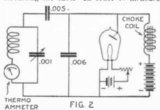
Circuit of a two-electrode tube for the production of radio frequency oscillations.
