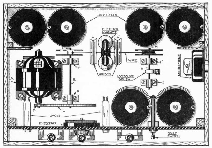
The telegraphone, the invention of Poulsen, the Danish Edison, embodies an electromagnetic phonograph in which a steel wire represents the disc, receives the message and delivers it over and over again if desired. The wire is seen towards the upper part of the illustration, passing between the poles of an electromagnet, which impresses the message and receives it again.
