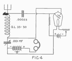
Another form of ultra-audion single control circuit. With the proper size honeycomb coil and variable condenser very good results may be obtained.
