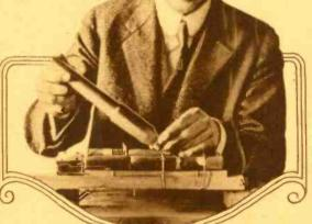
"Harnessing the electrons for heavy duty," is the keynote of Dr. Irving Langmuir's recent experiments in high power vacuum tubes, such as the 20kilowatt tube shown above. Marconi predicts that these tubes will replace the gigantic alternators now used for long distance work.
