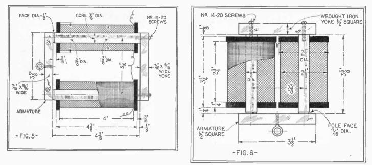
Dimensions with views are given of two powerful electromagnets, the first to be operated by a battery current, and the other one by a 110-volt D. C. lighting circuit. The first one, small as it is, can lift nearly 30 pounds.
