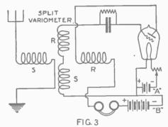
By using a split variometer a very good degree of both wave length and regeneration control is obtained with one knob. The efficiency of the circuit depends entirely upon the design of the variometer.
