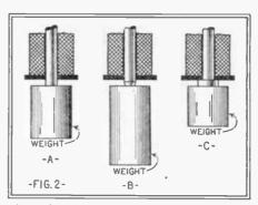
Examples of weights sustained by magnets with different shaped pole ends. For each case there is a certain shaped end which will give the greatest tractive power.
