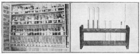
Left. A typical experimenter's chemical shelf. The guide-rails are wooden strips. The entire lower shelf is occupied by glass-stoppered reagent bottles. Right. A test tube rack can be easily made by the experimenter. Small holes in the top shelf support pipettes, stirring rods, etc. Use dowel rods for the pins.
