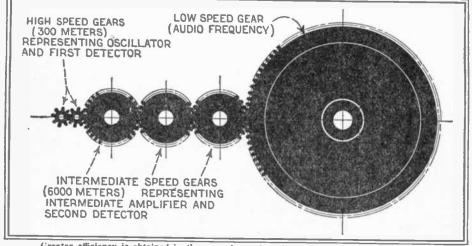
Greater efficiency is obtained in the super-heterodyne by employing an intermediate frequency amplifier, which in our analogy is represented by a train of intermediate gears. Note that as the size of gears change twice, two detectors are required.
