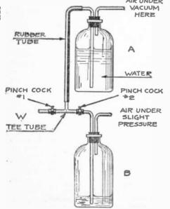
Fig. 1. Here's how to get water supply and air under alight pressure, even if running water is not available. Control is had by pinch-cocks (1) and (2). ness and speed of work and at the same time incorporates a semi-professional aspect at least. The few ideas in this article have been found very useful by the author in his work, and it is believed that they will be of advantage to many experimenters who contemplate starting a chemical laboratory.
