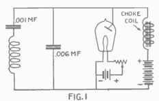
Circuit of a two-electrode tube for the production of audio frequency oscillations.
