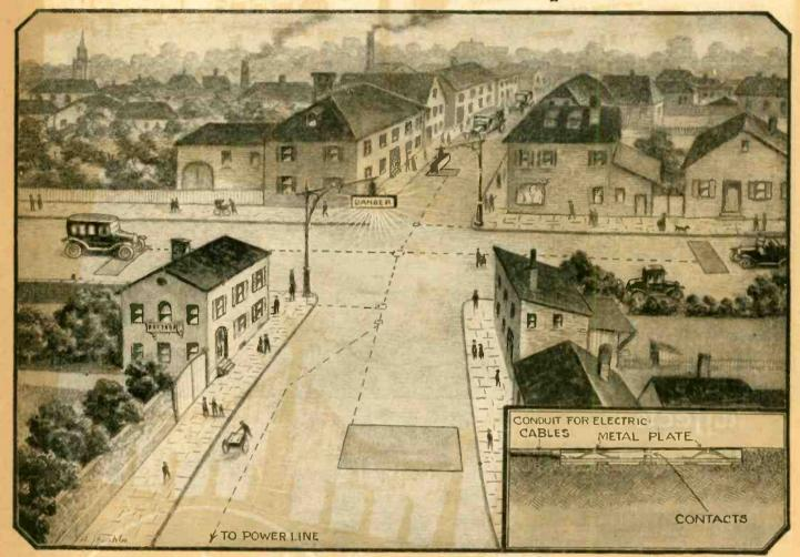
The latest evidence of electricity in the service of safety is this electric alarm at road crossings. Experiments performed at a dangerous cross-ing have proved decidedly successful. The pressure of the automobiles on steel plates set in the road a good distance from the crossings rings the alarm and flashes an electric sign, warning drivers on the other road of the approach of your car.
