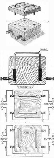
A simple reversing switch, which will prove a welcome addition to every experimenter's outfit. A sectional view of the switch, showing mercury contact wells is given; and below is shown the reversing switch hook-up.
