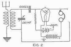
The ultra-audion type of single control circuit. Although no provision is made for controlling regeneration, with little experimenting the circuit may be adjusted to the point of maximum sensitivity without setting up oscillations.
