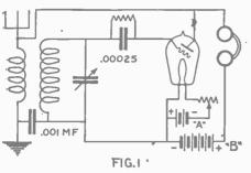
One form of single control circuit in which regeneration is obtained through the aerial or primary coil. By proper design and a little experimenting the circuit may be adjusted so as to hold the maximum value of regeneration throughout the entire tuning range.
