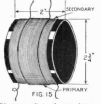
This air core radio transformer works very well in a reflex circuit when used in conjunction with a crystal detector. By tuning the coil with a 23plate variable condenser it covers the broadcasting range. It is used in many of the experimental circuits described.
