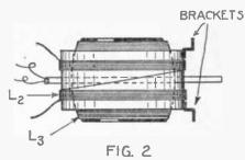
Showing the construction of the feed-back coupler, the details of which are given in the text. As it consists of two separate windings, it will be found useful in a variety of experimental circuits.
