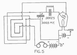
This circuit, worked out by Marius Logan, has very good possibilities. A tickler coil is incorporated in the loop, giving the desired degree of regeneration. Experiments so far conducted prove the circuit very efficient.
