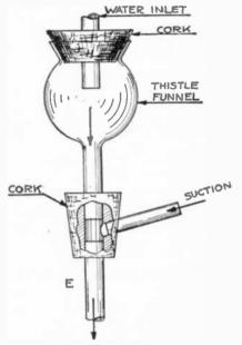
Fig. 2. A simple method for obtaining a vacuum. The parts here can be permanently installed or taken apart at an instant's notice, if they have to be used for other purposes.
