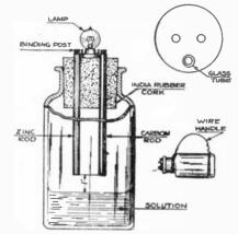
A novel electric torch with wet cell attached; the lamp is carried on the jar; the contact is closed by placing the jar on its side.
