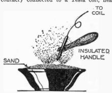
Try this spectacular eruption caused by a spark from a Tesla coil; the discharge causes sand to fly about as by a miniature lightning stroke.
