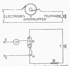
General connections of ear-phones and circuit breaker or interrupter, letters corresponding to the upper illustration. (G) is the grid. In every muscular contraction and also in every movement of a heart muscle there occurs a change in potential which can be transmitted by a conductor and indicated by a suspension galvanometer. In the electric organs of the electric eel these currents are also evident.
