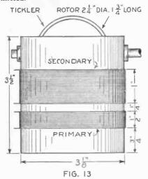
The experimenter can easily construct a homemade tuning coil by following these dimensions. This coil, comprising primary, secondary and tickler windings, may be used in many circuits.
