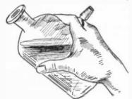
How to hold a bottle stopper when pouring out a chemical. The stopper must not touch the laboratory table, lest it should pick up impurities there.
