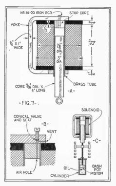
A so-called suction magnet; the core moves within a brass tube and means are provided for obtaining a dashpot action.
