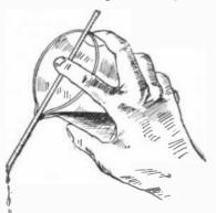
How pouring can be done with one hand. This is especially useful for small-sized beakers. For 500 cc. beakers and upward the first method is the best, and really the only one.
