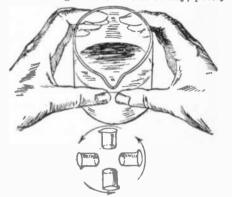
An odd way of pouring only to be used when the entire contents of a beaker are to be poured out. The beaker is turned completely around as shown in the diagram below.
