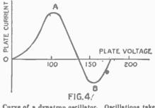
Curve of a dynatron oscillator. Oscillations take place when the voltage is adjusted between the values (A) and (B).
