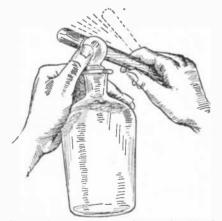
How to loosen a stopper when stuck; this plan is simpler than any other and works in the majority of cases. A wooden stick must be used, not a piece of metal, as the metal will break the glass.
