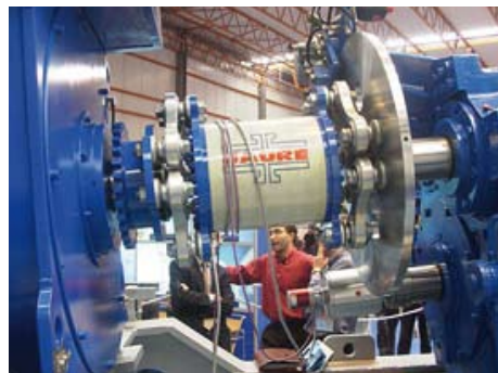
Ixilflex® with JGFS composite spacer.
