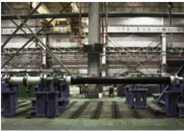
Carbon Fibre Shaft combined with LAMIDISC® coupling.
