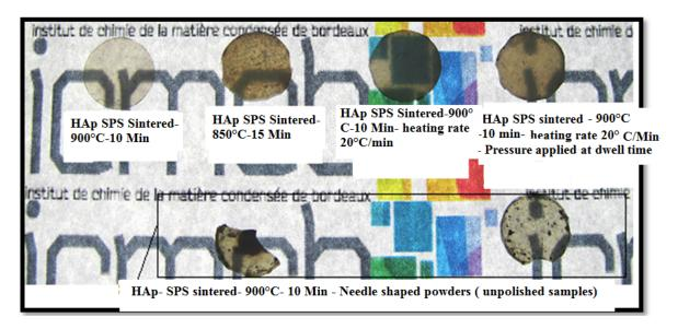
**Figure 7.** Fabricated transparent ceramics of hydroxyapatite with different grain morphologies.
