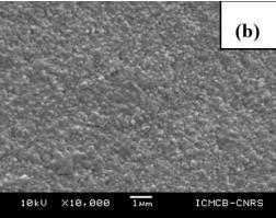
**Figure 6.** (a) Commercial HAp-SPS sintered at 900 °C, 10 min; (b) synthesized needle-shaped HAp-SPS sintered at 900 °C, 10 min.
