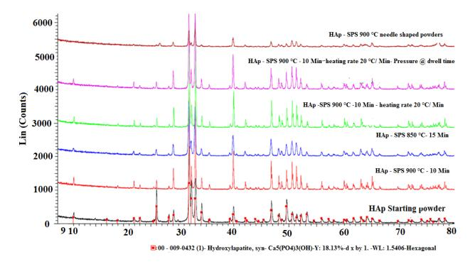
**Figure 5.** Comparison of the X-ray diffractograms of commercial HAp powders with a grain size of 50 nm and their sintered pellets in addition to HAp sintered pellets from synthesized HAp powders (~20 nm). SPS, spark plasma sintering.
