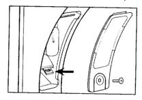
**STEP 3.** Remove the lens by pulling it down and away from drum.
