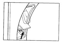
**STEP 5.** Remove the light bulb by turning it counterclockwise.
