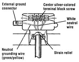
3-Wire Connection with Frame-Grounding Conductor
