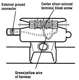
**STEP 5.** Connect neutral grounding wire and the neutral wire (white or center) of direct wire cable under the center screw of terminal block.
