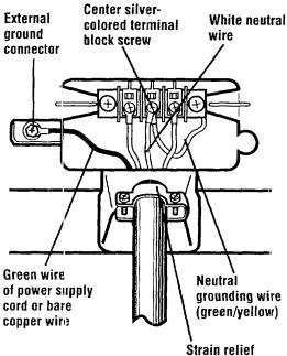
4-Wire Connection with Frame-Grounding Conductor
