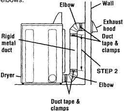
The duct usually comes in 2-foot lengths. Cut 2 inches longer than measurement for connection.
