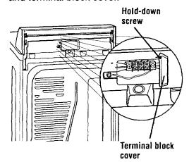
**STEP 3.** Attach <sup>3</sup>/<sub>4</sub>" U.L.-listed strain relief (U.L. marking on strain relief) to the hole below terminal block opening. Put the power supply cord through the strain relief.
