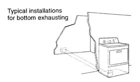
Avoid pushing the dryer tightly against a wall. This can crush or kink the duct. Use the straightest path you can, where possible, to avoid 90° turns.
