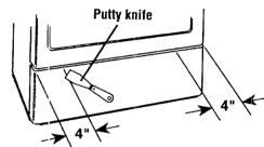
**STEP 3**. Remove lint from the dryer base with a soft brush or vacuum cleaner. Avoid damaging wires or electric thermostats.
