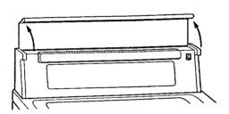
**STEP 3.** Pull off and remove the plastic light cover.
