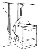
This dryer may be converted to exhaust out the right or left side or through the bottom. To convert the dryer, the following kits MUST be used.
