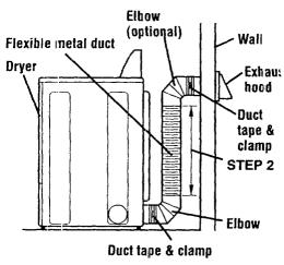
**STEP 2.** Measure the length of 4-inch flexible metal duct needed from the dryer to the hcod.
