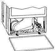
**STEP 4.** Replace lower front panel; reconnect and level dryer again, if necessary.
