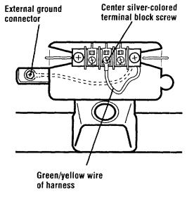
**STEP 5.** Connect neutral grounding wire and the neutral wire (white) of power supply cord under the center screw of terminal block.
