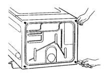
STEP 5. Now stand the dryer up. Slide dryer onto cardboard and move dryer close to its final location. Leave enough room to connect the exhaust duct.
