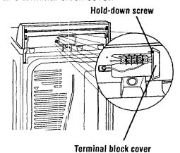
STEP 3. Attach 3/4" U.L.-listed strain relief (U.L. ma king on strain relief) to the hole below terminal block opening.
