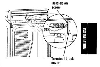
STEP 3. Attach <sup>3</sup>/<sub>4</sub>" U.L.-listed strain relief (U.L. marking on strain relief) to the hole below terminal block opening. Put the direct wire cable through the strain relief.
