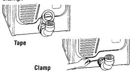
**STEP 4.** Connect rigid metal duct to elbow. Tape the joint with duct tape. Tighten clamp.
