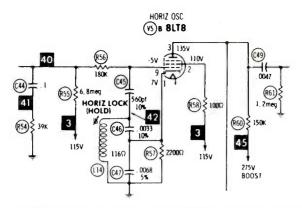
FIGURE 2. HORIZONTAL CIRCUITS IN ADMIRAL PK 1560.
