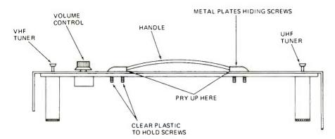
FIGURE 1. HOW TO REMOVE PLATE HOLDING TUNER AND VOLUME CONTROL ON-OFF SWITCH IN SOME ADMIRAL RECEIVERS.
