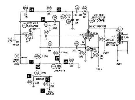
FIGURE 5. VERTICAL SWEEP, ARVIN MODEL 67K48.
