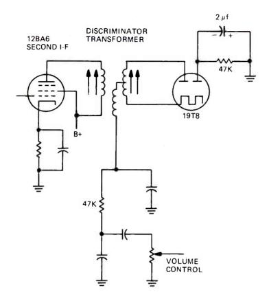
FIGURE 4. FM DETECTOR CIRCUIT IN PHILCO 50-925.
