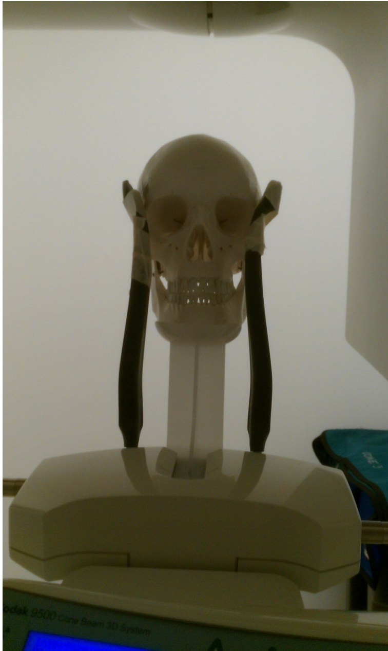
Figure 6. PVC model was mounted in similar fashion as actual patient during CBCT acquisition. Model was secured with adhesive tape.
