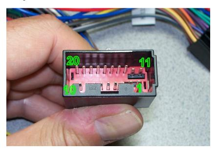
The photo above shows the harness side connector for the ISO harness. I also labeled the corner pins (the rest are in order). The harness also has labeled wires so you know what each one is. Below is the schematic for the standard sound system my car has.
