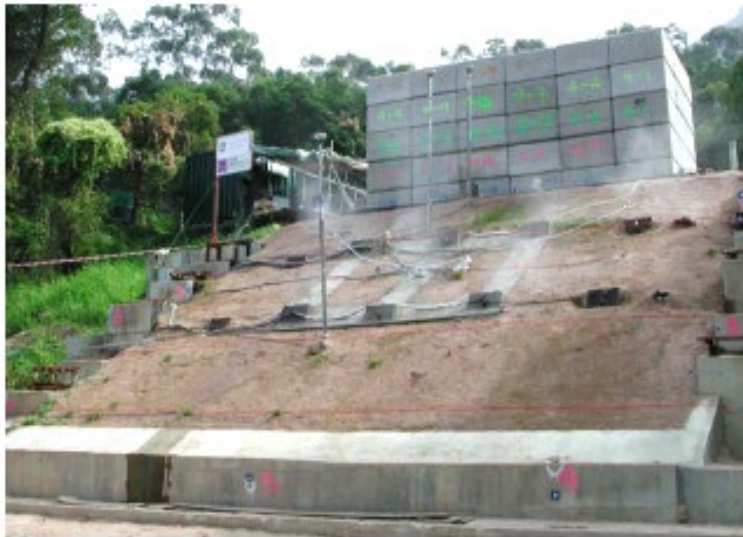
Figure 4. Loose fill slope testing with soil nails (Li et al. 2008).
