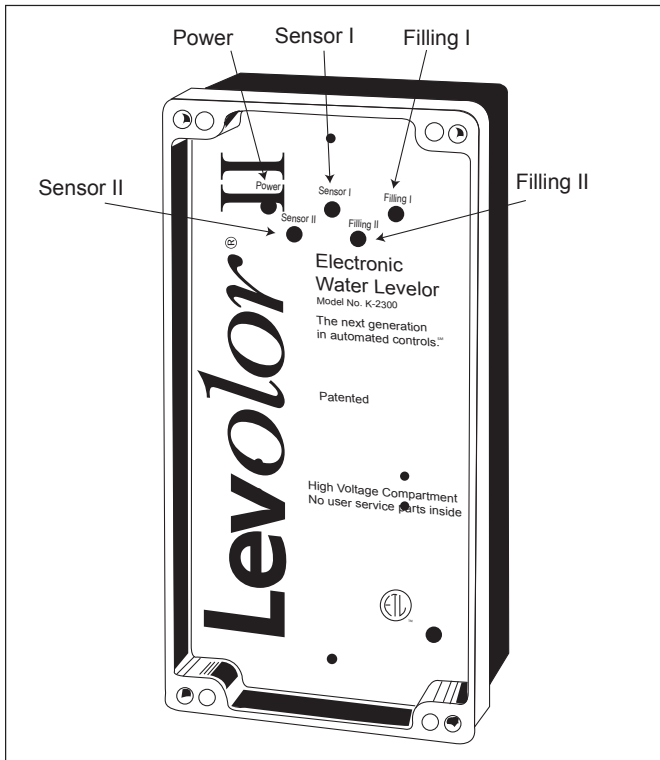
Figure 24. K-2300 Controller Lights
