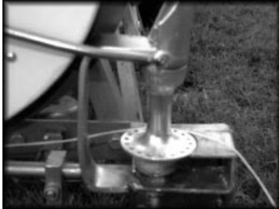
(left) Closeup view of the spindle when the bale is in the up position. Everything is shaped to prevent snags.
