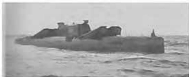
Juliett-class SSG with launching containers of P-6 missiles lifted for firing
