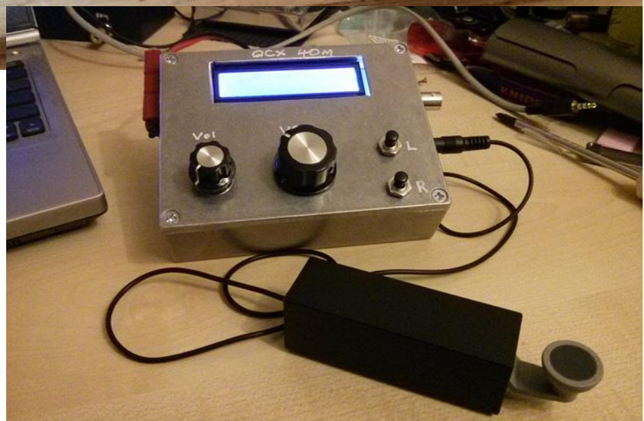
Palm PPK connected to the completed QCX:
