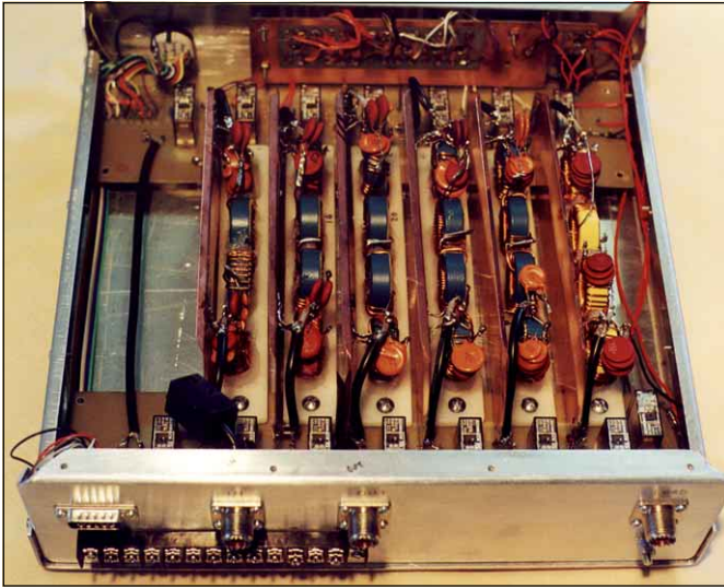
Figure 2—In the Mark I the filters and relays are mounted on open PC boards.
