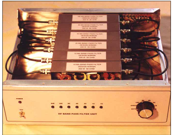
Figure 3—The Mark II filters are mounted within individual boxes.
