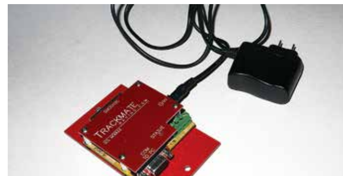
The interface board gets one of the two a/c power adapters. The power cable is about five feet long, so plan accordingly.
