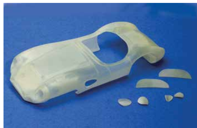
After taking it out of the bag, this is what we have. The Frosted Ultra Detail printing material is pretty see through in some areas. There is very little stepping on the printed body. The first thing you have to do is to degrease it. Acetone is recommended, as it will cut through all the leftover oils and what nots that were used in the printing process.
