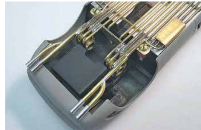
Brass tabs were soldered to the rear of the chassis just ahead of the front wheels, for body mounting. Plastic tubes were added to the inner fenderwell and a brass threaded ferrule provides the threads to seat the screw tightly.
