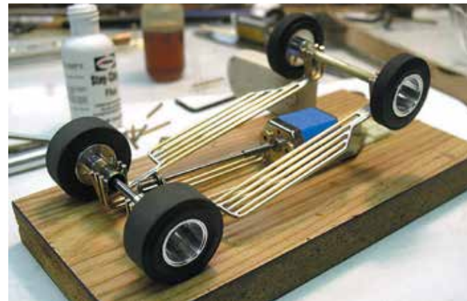
Demonstration of the ISO pivot. After the limiter is in place the movement will only be 1/16" up or down. The pivot is the axle tube itself.
