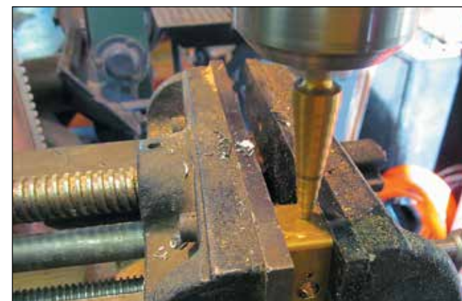
For anyone wanting to run 1/8" axle bearings or wanting to install an axle tube, there is plenty of meat on the bracket for milling. For me, I wanted to run more than one bearing per side, so installing an axle tube was necessary. A step drill made quick work of opening up the hole to fit 1/4" tubing.
