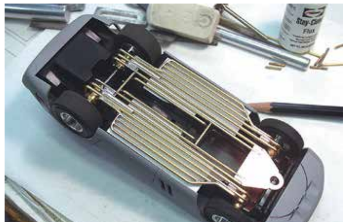
Chassis test fit into the body shows that clearance will need to be cut into the front valance to provide room for the guide and lead wires to swing back and forth.
