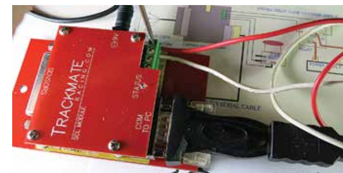
The red and white wires from the relay attach to the TrackMate Interface board. The black cable on the bottom right is the cable to the computer, via the serial to USB adapter.
