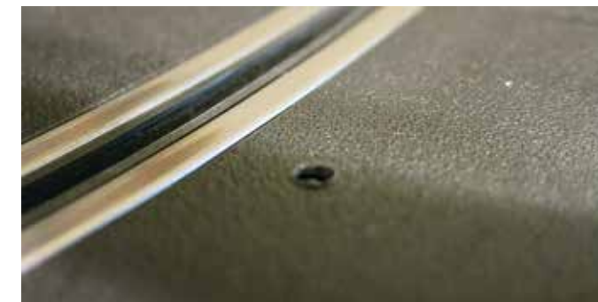
You can barely see the tip or head of the infrared sensor. The instruction manual says to chamfer the top of the hole you drilled (the 1/8" one), with a drill bit a couple of sizes bigger, to give the sensor a better and wider field of view.
