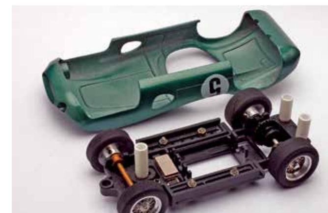
For the body mounts, we used the Slot Car Corner body mounting kit, the shortest one. The styrene tubing was measured for length by running a toothpick through the screw hole opening up to the underside of the body, and marking the toothpick, allowing for the thickness of the chassis. It was a hit-and-miss kind of thing, but we can't think of a more accurate way of doing it.
