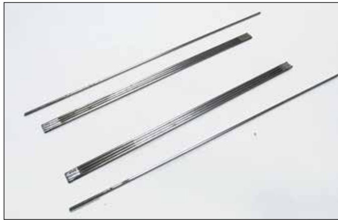
Two sets of .047" rail clusters are soldered together. The outside fifth rail will taper out, forming a triangular shape to hang the pans from. This triangle will also keep the chassis from flexing side to side.
