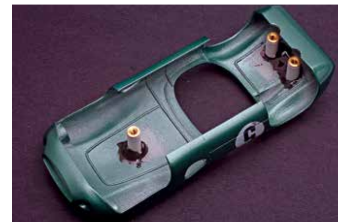
After letting the J-B Kwik Weld dry for about 15 minutes, the mounting screws were removed. It looks kind of sloppy, but it gets the job done. Maybe next time we will get better with the gluing of the body mounts.
