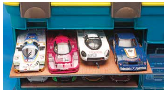
We made the shelves to slide right into the rails in the box. We drilled out four grooves to accommodate the slot car guides. We should have used a router to create more even grooves.
