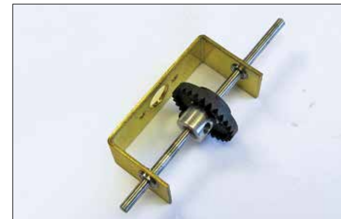
The rear bracket is already set up wide so no axle tubes are usually needed. 3/32" bearings pop in and are ready to go! But I have broken these bearings with one wall shot. I feel the need for better bulletproofing!
