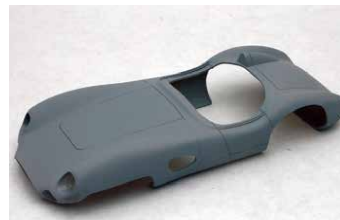
After cleanup, making sure there were no oils or anything left on the body, it was lightly sanded with #400 grit sandpaper. It only took a few lights passes of sandpaper to get it ready for paint. That's what we like about the Frosted Ultra-Detail material. The detail is so much better, and the printing "steps" on the body are a lot finer. A quick primer coat showed we had a few more areas to sand and clean up. We like to use a lacquer primer/surfacer for this stage.
