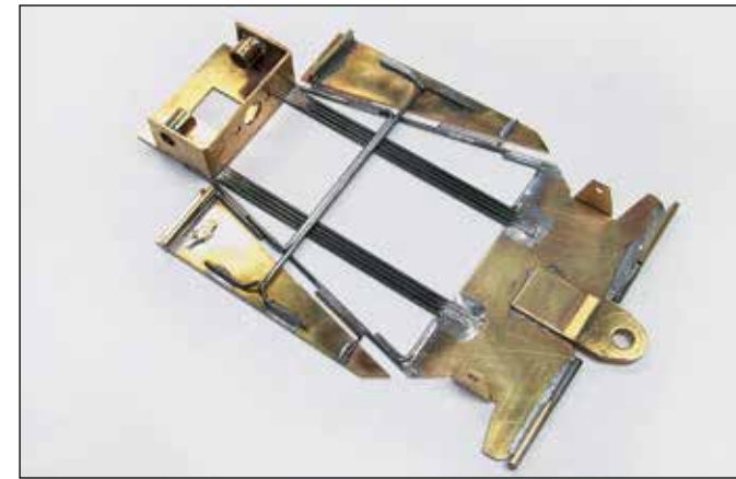
Here the chassis has been cut away for the front wheelwells. Also installed is a set of .078" steel front bumpers in order to keep the forward pan from bending. Above that I installed a 1/16" brass tube for the forward body mount.
