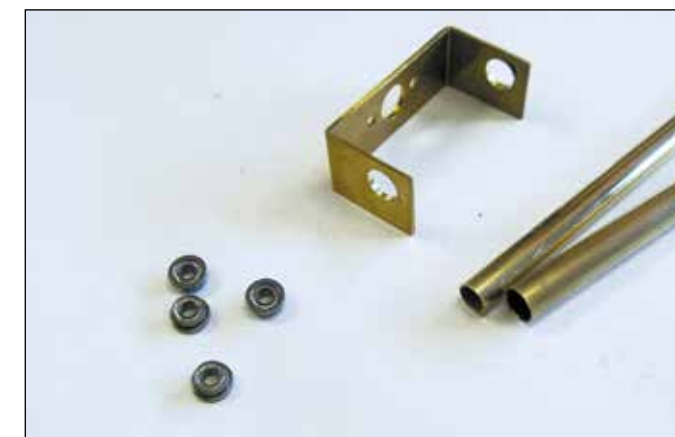
Two tubes (1/4" and 7/32") were inserted into the holes, soldered together and to the bracket, before cutting. This provides lots of support for any wall hit and reduces the chance of a bent axle or broken bearing down to nil.
