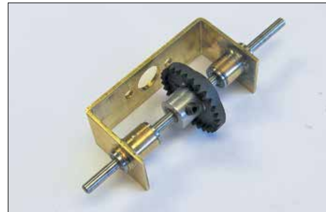
Now we have something solid enough to withstand the rigors of racing! The crown gear is a 48 pitch, 28 tooth Parma product. It was supplied through PCH Parts express. While it comes molded in pink, PCH sleeves them for the 3/32" axle. This is a popular Retro item used by nearly all the pros because they are straight and can be found in 29 and 30 tooth for tuning. The reason it's black here is because I dye them in Rit dye.
