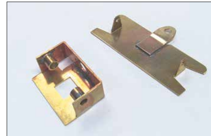
A piece of .040" brass plate is added to the bottom of the bracket, which was originally set up for .78" diameter rear wheels. This car will use .87" Protrack rears, necessitating raising the axle centerline. The plate also adds needed weight and strengthens the bracket. It also provides a nice flat area to place lead handling weight, if need be.
