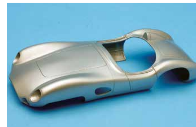
After the primer was smooth and the body not showing any imperfections, it was time to lay down a base coat of silver. We like to use silver, as it gives you a very good bottom color for your top coats. This is Tamiya Bare Metal Silver.
