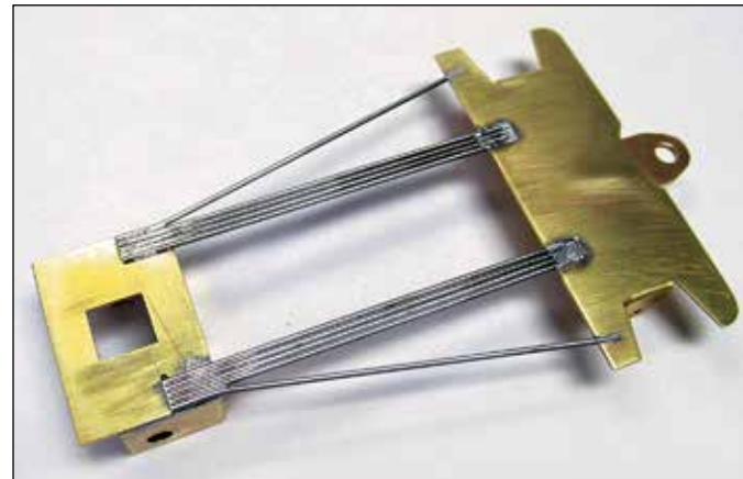
Here is the completed center section right off the jig, top and bottom. At this point the flex is good enough for most any track. However, if the chassis proves to be too flexible, adding solder to the rails will stiffen them considerably, so some tuning is possible. Likewise, adding weight is very easy since I have kept lots of flat areas free to stick the lead sheet to. At this point we have a chassis strong enough to drive nails into the wall.
