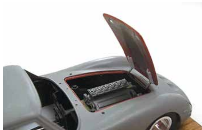
Engine compartment details will be clearly visible with the hood opened. Magnets allow the hood to stay open with no prop rods required.
