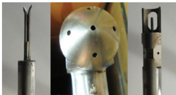
Three types of pitot probes. From left to right: s-probe, spherical probe, prism probe. Credit: NIST
