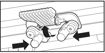
Figure 13. Seat Height Adjustment - Seat Latch Safety
