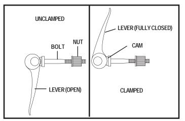
Figure 19. Quick Release Fastener Operation
