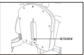
Figure 20. Bottom View of Foot Platform
