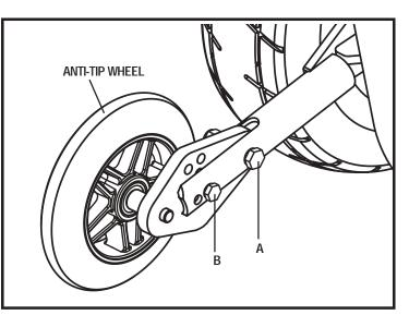
Figure 21. Anti-Tip Wheel Assembly
