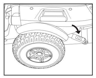
Figure 9. Freewheel Mode (Drive Disengaged)
