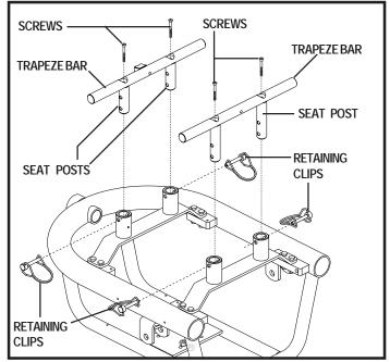
Figure 14. Seat Height Adjustment - Trapeze Bars
