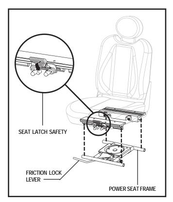
Figure 12. UMS - Power Elevating Seat System
