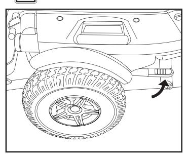
Figure 8. Drive Mode (Drive Engaged)
