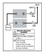
Battery Set Configuration: + = Positive (Red) Terminal Post - = Negative (Black) Terminal Post Connect Red wire to Red Positive (+) Terminal Post Connect Black wire to Black Negative (-) Terminal Post
