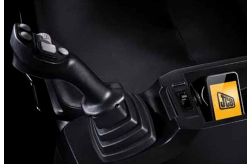
Optional multi-function joysticks enable the operator to operate a wider variety of hydraulically driven attachments. The left arm rest also features a storage compartment.
