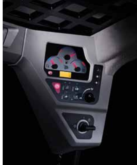
The right control panel features machine diagnostics, an electronic throttle and the ignition.
