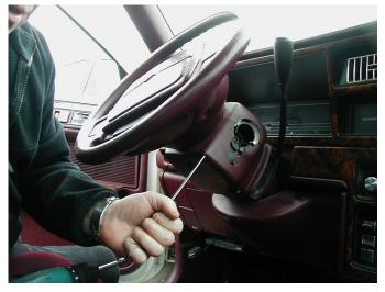
3) All of these screws should be 20 torx. The covers snap together closer to the dash and can be pulled apart after all the screws are removed.
