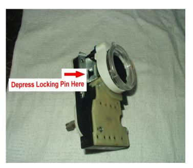
Once depressed, the lock cylinder will slide out of the switch.
