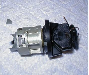
If the lock cylinder is broken (as illustrated) make sure you locate and remove the broken piece from inside the switch to avoid an electrical short.
