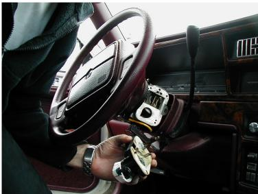
Lower the switch assembly to remove the wire connectors.
