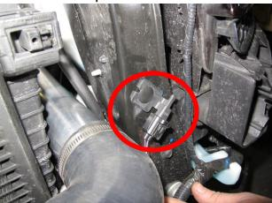
Step (25): Install coolant over flow bottle
