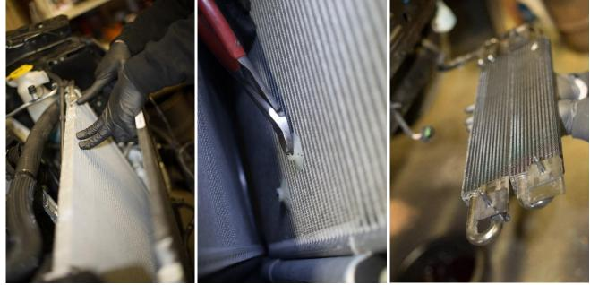
Mount trans cooler as shown (Must be mounted below bumper beam to fit intercooler) - reinstall white • retainer clips on back side of A.C. condenser
