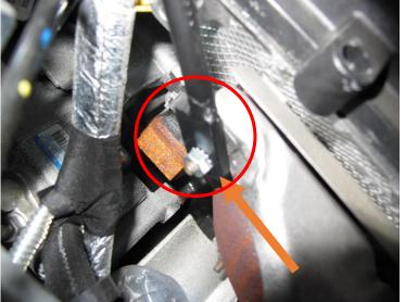
Bottom is over sized hole for final adjustment Tighten Second
