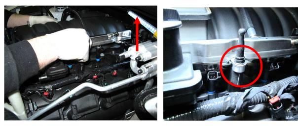
**Step (5) Install Spark plugs:** This kit comes with 16pc NGK Spark Plugs in a one-step colder configuration they will need to be gapped down.
