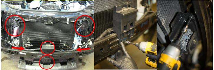
• Remove horns, bracket, and cruise control module and set aside (will be reinstalled later)
