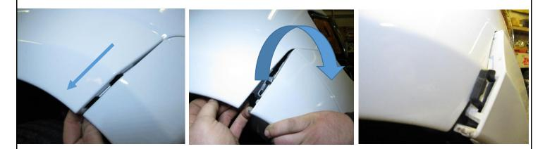
Gently pull the fender toward you with controlled force to separate the locking tabs that connect the bumper to the fender. Hold the fender and the bumper and push the bumper in towards the vehicle while also pulling down in one motion. You will hear a popping sound once bumper is free, this is normal.
