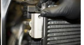
Detach Automatic Trans Cooler from A.C. • Condenser (Fig 4) Let hang freely
