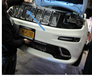
Note: Twist to unlock slowly on the Air Temp Sensor and straight as it will break coming out on an angle - THIS WILL BE REUSED IN LATER STEPS
