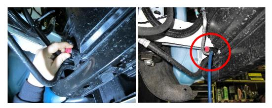
**Step (7): Remove upper coolant hose** from driver's side of radiator and cut approximately 2.25in off the radiator side of the hose or to the first bend FIG 1. This will make room for the supercharger installed in later steps. At this point please bend hose away from work area as per last picture. In later steps you will be reusing the factory clamp.
