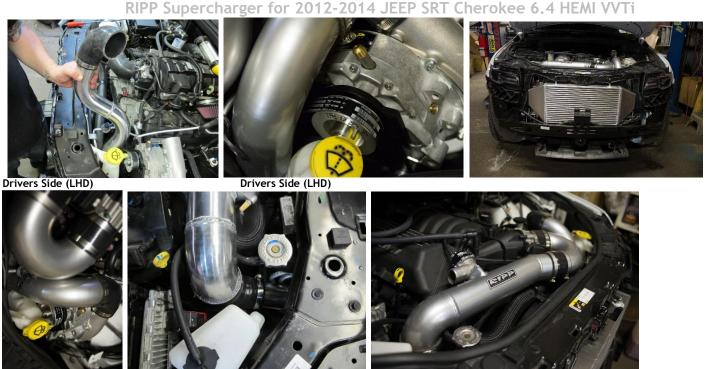
Passenger Side (LHD) may have to bend the A/C Line slightly too clear using same technique as drivers side (LHD) \* Place 3.5in to 3in 90deg Coupler to Pipe 3 and finally place Pipe 4 180deg pipe on Throttle Body
