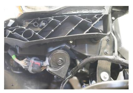
• Separate horn wires from factory harness and shielding
