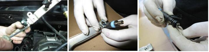
Use a flat-head screwdriver to pull back injectors locking clip
