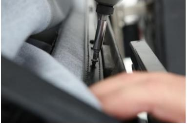
**Step 2 Snap top to rear bow**Raise the header and bow assembly toward the windshield and into position.
