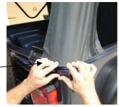
Step (6): Close the header latches to secure the front of the top to the windshield. Catch the hook in the slot in the windshield frame and then close the lever over it so that it lays flat against the windshield frame.
