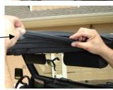
Step (11): Close the zipper on the quarter panels the rest of the way to the lower rear corner of the panel.
