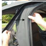
Step (10): Locate the plastic strip sewn to each side of the top, above each door. Slip the strips into the channel in the door surround above the door opening.
