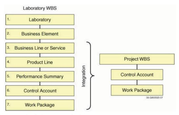
Figure 1. Integration of Laboratory WBS and Project WBS
