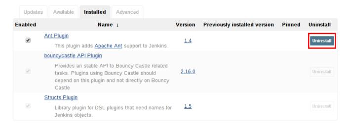
A plugin may also be uninstalled by removing the corresponding .hpi file from the JENKINS\_HOME/plugins directory on the master. The plugin will continue to function until the master has been restarted.
