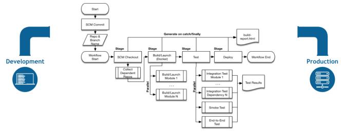
Figure 2. Pipeline Flow
