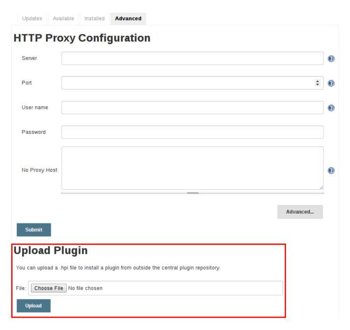
Once a plugin file has been uploaded, the Jenkins master must be manually restarted in order for the changes to take effect.
