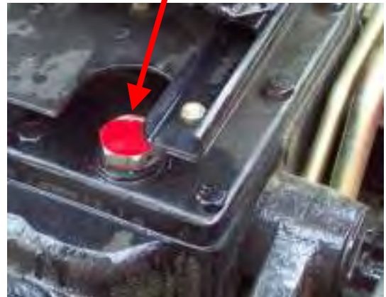
Hydraulic Fluid Fill
