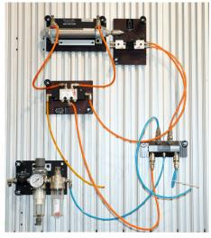
PneuFlex components mounted on the training panel
