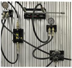
HydraFlex components mounted on the training panel
